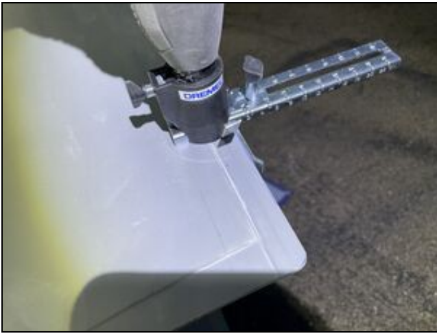
Squaring the joggle step with a dremel set to 0.75 inches and the joggle depth.
