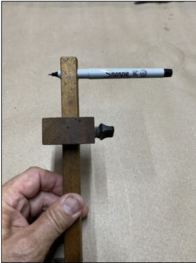
Carpenters Scribe Modified for sharpie
